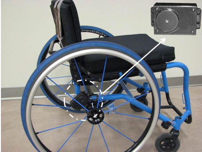
Figure 1: G-WRM attached to the spokes of a manual wheelchair.
